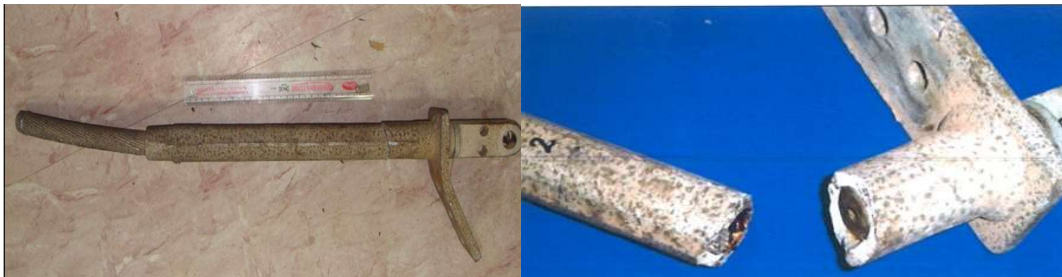
Dead End Fitting of TL –Point/Location of Conductor Snapping
