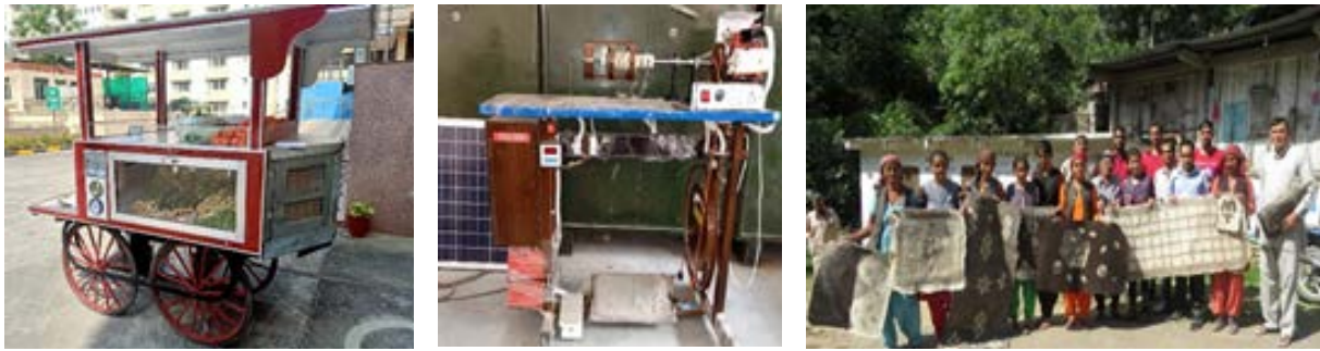
Figure 1: from left a) Air cooled vegetable vending machine b) Variable Speed Solar Based Bageshwari Wool Charkha c) Mechanised Roller (Felt Making Machine)
