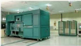
Combined bi-axial vibration and environmental test equipment
