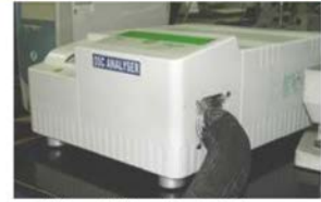
Differential Scanning Calorimetry (for Thermal analysis)
